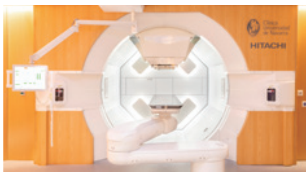
A proton therapy system at the Clinica Universidad de Navarra in Spain (the first system Hitachi has delivered in Europe)
