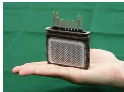
Direct water-cooling type double-sided cooling power module
