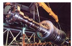
High-efficiency 600°C-class high-pressure turbine for thermal power generation
